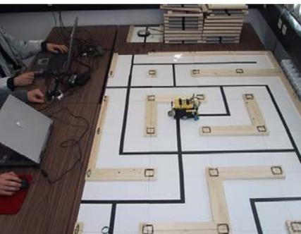
A wooden maze (*physical part of the scenario*, left) which is built with low-cost components and usage of Lego RoboLab
