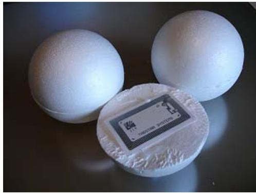
**Figure 2** RFID tag inside
