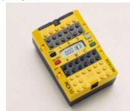
**Figure 1 - The programmable Lego brick RCX**
